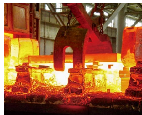
硅钢板在加热炉中加热 Silicon steel plate is heated in heating furnace
